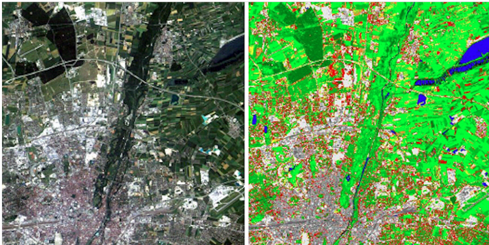
Figure 4.83: Example of classification with SPECL. Left: true color image of Landsat TM, right: result of classification.
