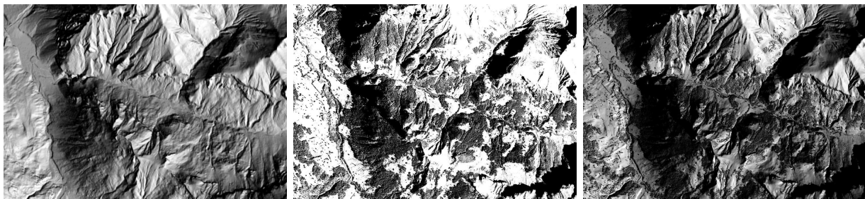
Figure 13.4: Combination of illumination map (left) with cast shadow fraction (middle) into continuous illumination field (right).
