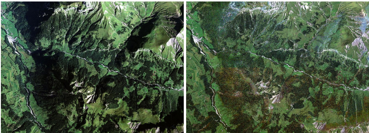
Figure 13.6: Effect of combined topographic / cast shadow correction: left: original RGB image; right: corrected image (data source: Leica ADS, central Switzerland 2008, courtesy of swisstopo).
